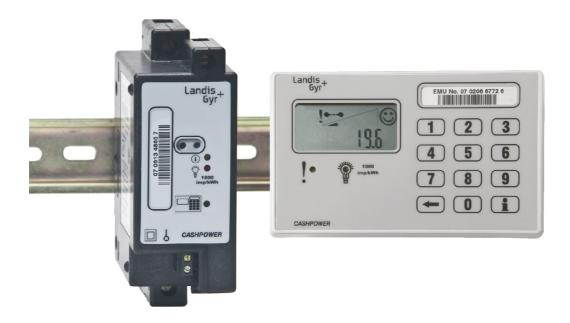
Cashpower Power-Rail is a single-phase 60A (80A optional) split meter in a DIN rail-mount housing. It is ideal for new reticulation where housing is informal with the prepayment meters mounted in a pole-top enclosure with respective customer interface units conveniently mounted in the dwellings below.
